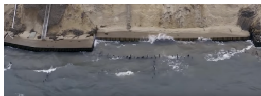
Past armoring fails and the debris continues to degrade the shore and beach. (All photos: MLive.com)
